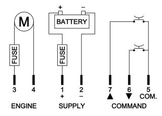
ELECTRONIC CONTROL UNIT FOR END OF STROKE CONTROL OF THE PE40G AND PE40GE ELECTRIC PISTONS.
