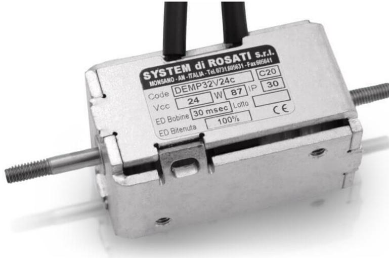
Bistable electromagnets have built-in permanent magnets and are suitable for safety systems that require operation independently of the power supply, as they maintain their position without voltage, making them ideal for battery operation or continuous duty applications.
