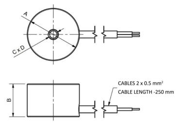
THE HOLDING FORCE IS A FUNCTION OF THE OPERATING TEMPERATURE, THE QUALITY OF THE CONTACT BETWEEN THE ELECTROMAGNET AND THE HOLDING PAD AND THE TYPE OF HOLDING IN RELATION TO THE THICKNESS, E.G. THE INDICATED RELEASE HOLD, SLIDING HOLD, ROTATING HOLD FORCES ARE REFERRED TO A RELEASE HOLD, WITH A SINGLE WORK CYCLE AT A TEMPERATURE OF 20°C AND WITH A HOLD PART 6 mm THICK WITH A DIAMETER EQUAL TO THE ELECTROMAGNET'S EXTERNAL DIAMETER.
