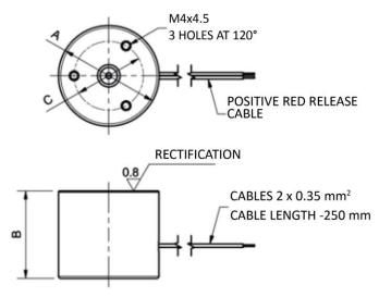
NOTE THE RECTIFIED SURFACE BEING FREE OF GALVANISATION. IT MUST BE KEPT LUBRICATED IN ORDER TO AVOID OXIDE FORMATION
