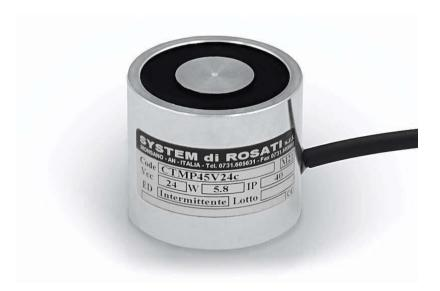
Holding electromagnet with permanent magnet type CTMP exerts an attraction force when not energised. The attraction force is in fact generated by the integrated permanent magnet and release is achieved by powering the electromagnet, which generates an electromagnetic field of reverse polarity.
