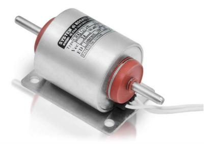
Rotating electromagnet type CR with single coil with 45° max. rotation angle, high rotation frequency max. 20 Hz. This high-frequency rotating electromagnet can be used for continuous ED duty=100% or for customised duty cycles.
